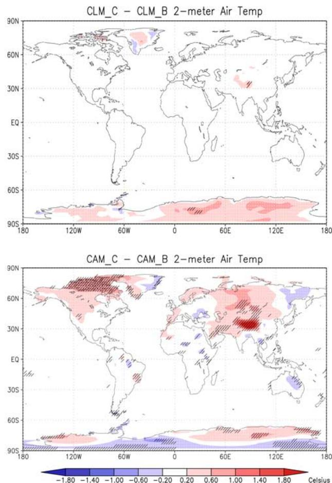
**Figure 2.** Climatological annual mean difference in 2 m air temperature caused by sub-surface snowpack solar absorption (top) in an off-line land model and (bottom) in a coupled land-atmosphere model. Hatching shows regions where differences are statistically significant at the 1% confidence level.
